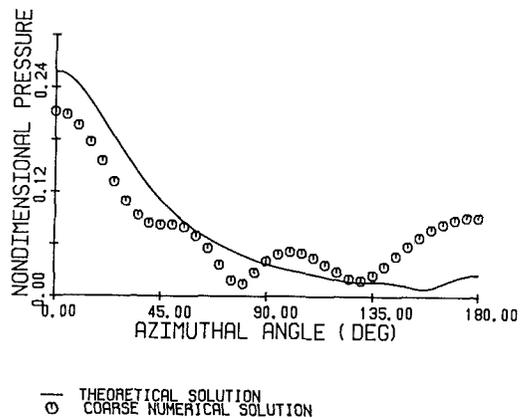
**Fig. 7 Radiated nondimensional acoustic pressure versus  $\phi$  for the case of the piston set in a sphere; coarse model;  $ka = 5.0$ ;  $r/a = 2$**
