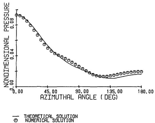
**Fig. 6 Radiated nondimensional acoustic pressure versus  $\phi$  for the case of the piston set in a sphere;  $ka = 2.0$ ;  $r/a = 2$**
