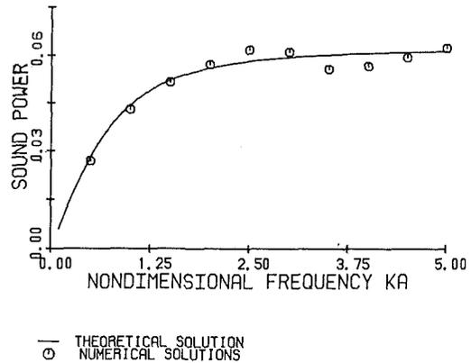
**Fig. 9 Total radiated nondimensional sound power versus  $ka$  for the case of the dilating sphere**
