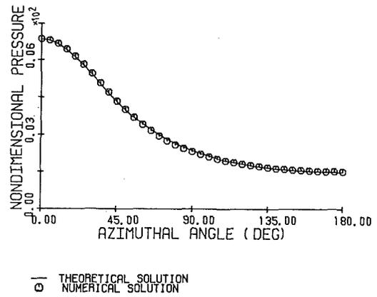
**Fig. 5 Radiated nondimensional acoustic pressure versus  $\phi$  for the case of the piston set in a sphere;  $ka = 0.02$ ;  $r/a = 2$**
