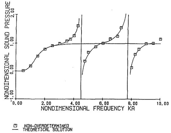
**Fig. 3 Nondimensional surface pressure versus  $ka$  for the case of the oscillating sphere;  $\phi = 0$**
