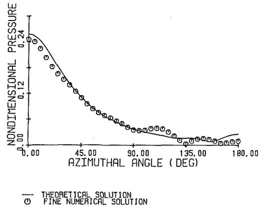
**Fig. 8 Radiated nondimensional acoustic pressure versus  $\phi$  for the case of the piston set in a sphere; fine model;  $ka = 5.0$ ;  $r/a = 2$**
