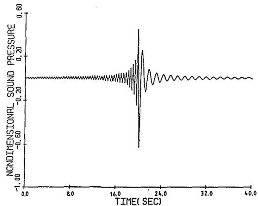
**Fig. 10 Temporal acoustic response—Doppler effect  $ka = 1.0$ ,  $c = 1.0$ ,  $v = 0.5$ , stationary dilating sphere**
