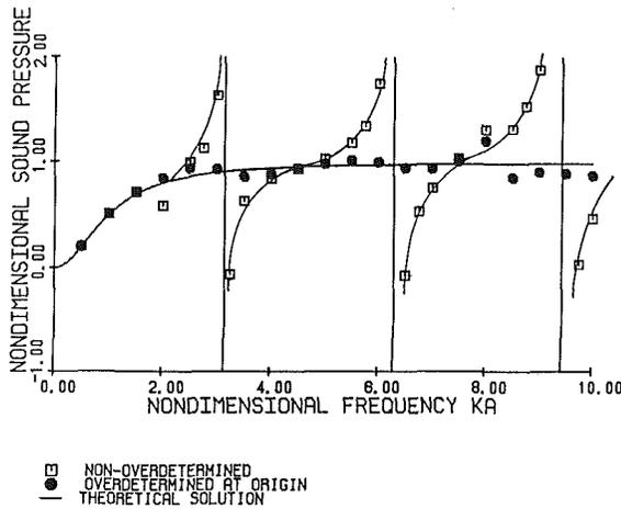
**Fig. 2 Nondimensional surface pressure versus  $ka$  for the case of the dilating sphere**
